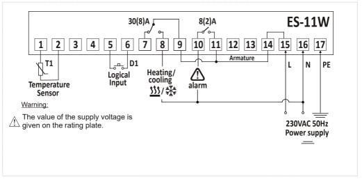
Connect the connecting cables through the cable glands and tighten them firmly to obtain a full tightness of the gland. Secure the wiring harness with clamping sleeves. The screw terminals of the controller allow connection of a cable with a maximum cross-section of 4mm2.
