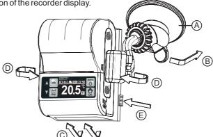
Turn the knobs so that the handle doesn't unlock and doesn't move while driving. After some time of use, re-tighten the knobs and tighten the clamping jaws and make sure that the recorder is properly mounted.
