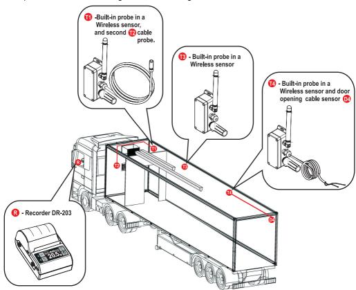
Thanks to the built-in thermal printer, you can document the temperature registration process during transport and provide a report for the recipient of goods or control services. DR-203 allows you to print three types of report:
