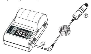
First insert the car charger (F) into the cigarette lighter socket. The charger power LED will light up. Then insert the miniature round plug into the power socket (G) on the right side of the recorder. The device is ready for work. To turn on the recorder press but a name of the recorder press b
